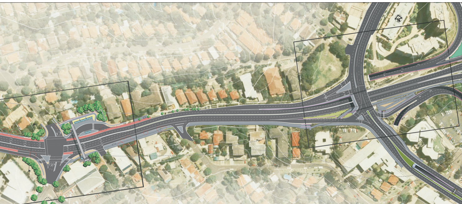
cyclists, pedestrians and public transport. The section shown here, between Centennial Avenue and the Pacific Highway, now has a narrower roadway with bus lanes and a cycleway.
