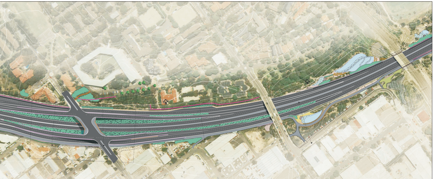
ramps and shared cycleway and pedestrian path between Naremburn and the eastern portals of the Lane Cove Tunnel and the Pacific Highway and Longueville Road (left).
